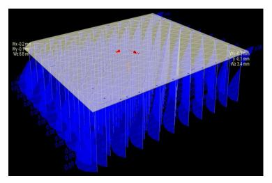
From the three pictures above, it can be summarized that the maximum bending moment that occurs is 0.40 kN.m while the quality of the minipile is able to restraint the bending moment of 35.4 kN.m so it can be concluded that the bending moment number that occurs is still below the bending moment that it can restraint by the minipile. Meanwhile, the settlement rate that occurs is 6.8 mm or 0.68 cm, which is still smaller as required by the design criteria, which is a maximum of 2.5 cm.
